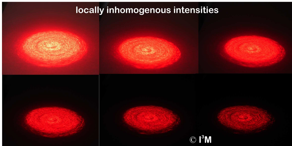
Fig. 3: Locally inhomogeneous intensities in a laser beam. The respective pictures represent different integration times.
